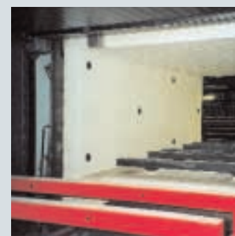
Shuttle kiln with lift carriage for the ceramic industry
