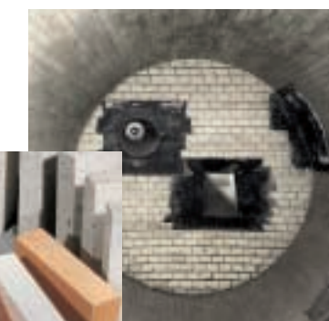
Rotary melting furnace for the aluminium industry
