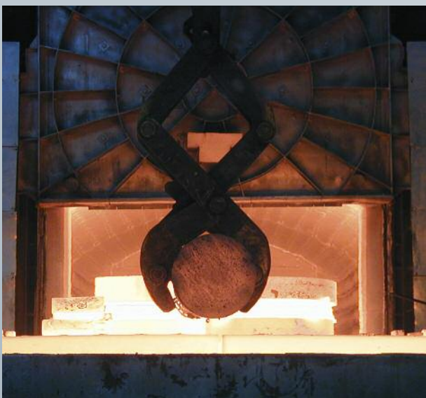
Annealing forging in front of bogie hearth furnace
