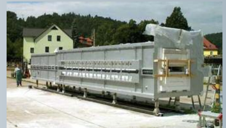
Pre-assembly of a continuous pusher-type hardening furnace
