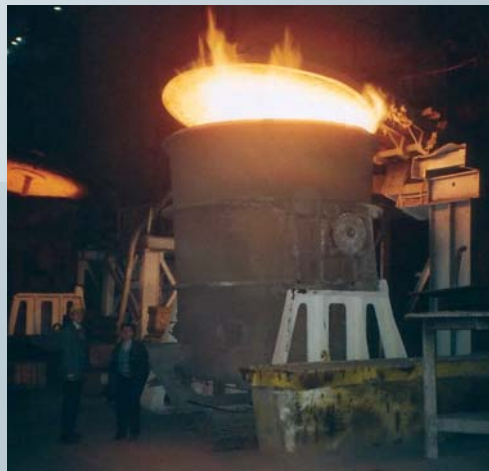
Heating of a steel casting ladle
