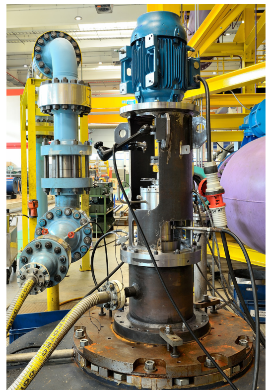
VS1 pump ready for performance test
